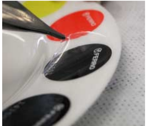
Fig. 3: Removal of the strippable coating 80 2039
